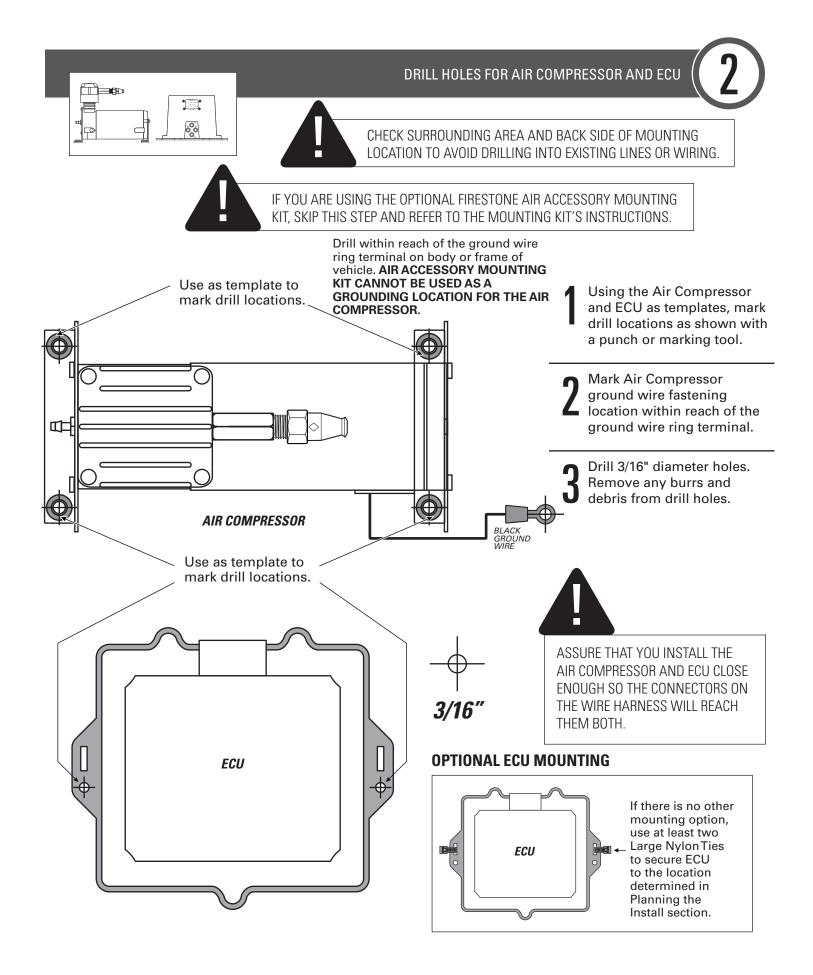
INSTALL THE AIR COMPRESSOR AND ECU
