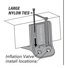
2 Select a protected location to install the Inflation Valve, such as the bumper or the body of the vehicle.
