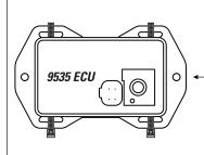
If there is no other mounting option, use two Large Nylon Ties to secure ECU to the location determined in planning the install section. Route the Nylon Ties under the ECU and around the mounting location.
