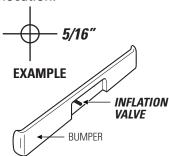
Install Inflation Valve Assembly as shown.
