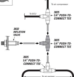
2 Cut the piece of Air Tubing that connects the two installed 1/4" Push-to-Connect Tees.
