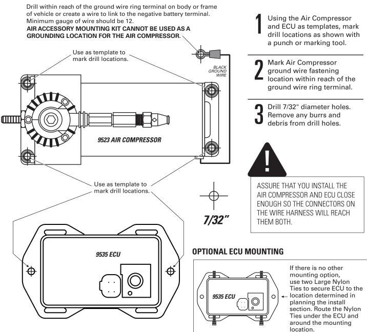
INSTALL THE AIR COMPRESSOR AND ECU
