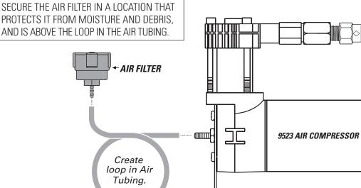
AIR LINE TUBE FROM AIR COMPRESSOR KIT
