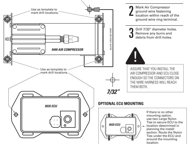
INSTALL THE AIR COMPRESSOR AND ECU
