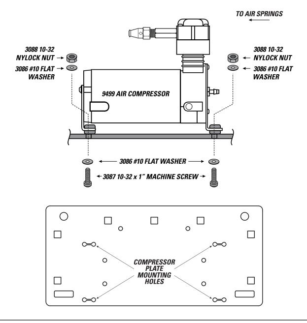
AIR ACCESSORY MOUNTING KIT CANNOT BE USED AS A GROUNDING LOCATION FOR THE AIR COMPRESSOR
