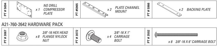
Mount the No-Drill Compressor Plate to the Plate Channel Mounts shown below.
